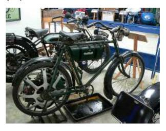
The Singer Motor Wheel looks very much like a forerunner of the Cyclemaster with its engine and fuel tank carried entirely within the rear wheel (the in-frame tank on this one is an auxiliary; the normal tank is in the wheel and also acts as a surface carburetter). It's not really a true cyclemotor because it has to have a special frame. Not only do the forks have to be extra wide to fit around the engine, but they also have special fork ends to fit the Singer's axle.
