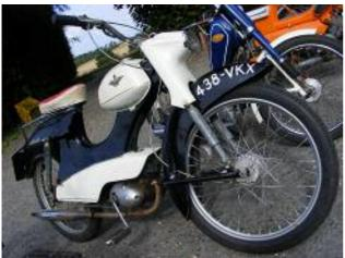
On the other hand, this is nothing like as old as the Wall Auto Wheel, but is much rarer. It is an **Ambassador Moped** dating from 1961. Although powered by a Villiers 3K engine, the cycle parts didn't originate in the UK Kaye Don's Ambassador company imported most of the machine from Solifer in Finland. As well as fitting the Villiers engine,
