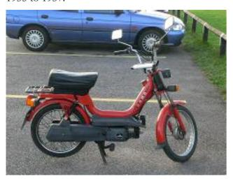
The Garelli Como first came to these shores in July 1985. A typical 'Europed' with its oversized frame tube doubling as a fuel tank, the Como was a single-speed automatic 49cc machine with front and rear suspension. The Como 2, a two-speed version, came in September of the same year. Both the Como and the Como 2 were also available in De Luxe forms. The only difference was that the De Luxe had flashing indicators.
