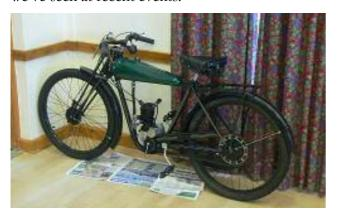
Here's a bike that attracted a lot of interest at Kneel's Wheels: Luke Booth's Peugeot. It's a typical French BMA (Bicyclette à Moteur Auxilaire - the French equivalent of our autocycles) of the 1930s. Very simple and - as Mick Cook can verify - very light. Peugeot produced quite a range of these machines during the 1930s and we reckon that this one, with its spring forks and drum brakes, is near the top of the range: a P50T from 1935 to 1937.
