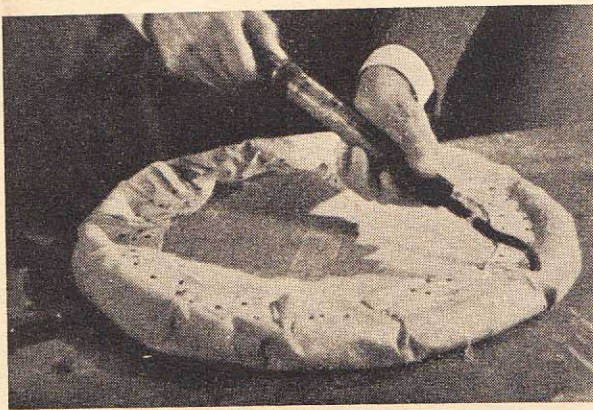
A reproduction of the first Dunlop tyre. It was made from thin sheet rubber, blown up with a football pump and attached to a wooden disc with a strip of linen.
