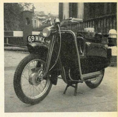
tool and or glove compartments on either side of the rear wheel. All these panels are spring loaded and shut securely without rattles or fiddly clips.
