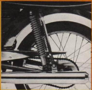
Rear suspension by swinging fork with new double-spring hydraulic shock absorbers. Secondary transmission with very efficient torque-damper. New exhaust-pipe, very modern style, with approved exhaust-gas silencer. New design chain-cover. New tail lamp with increased reflex-surface. Comfortable new cushioned seat of high quality. BRAKES: 105 mm. (4.1 in.) diameter. TYRES (FRONT & REAR) 2.25 x 18"
