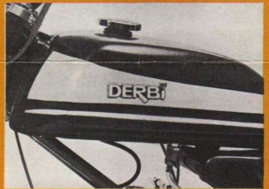
New style fuel-tank large capacity, in red and white metal painting, furnace hardened. New fuel-tank cap.
