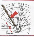
Place the driving belt round the rim, and refit the rear wheel; adjust the chain tension in the usual way. Tighten the extension bolts. The driving rim must now be trued up in position before tightening the clamping screws. This can best be done by making a chalk mark on the bottom stay tube about 72 inches from the hub spindle. Rotate the wheel and gently tap the rim until it runs true in relation to the chalk mark, tighten up the clamp screws all round the rim.
