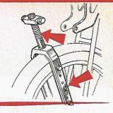
Remove the existing rear spindle nuts which will not be required. Fit the extension bolts supplied with the motor. These are hollow to accommodate a 3-speed control if one is fitted.
