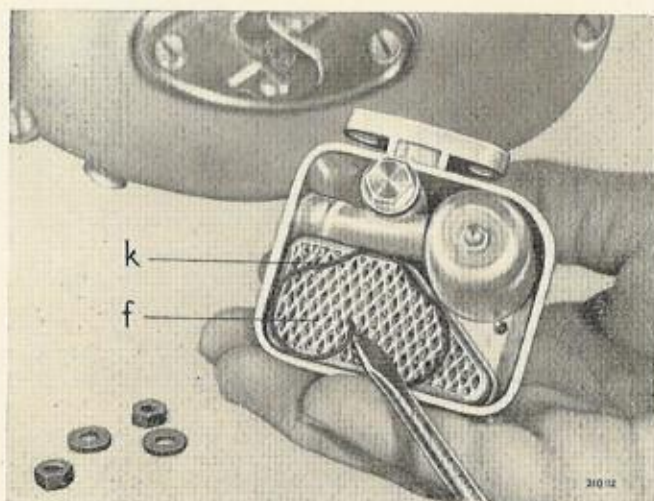
Fig. 7. Air Filter in Carburettor. f—Filter element. k—Spring ring.
