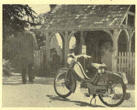
EXTENSIVE shielding and deep, effective mudguarding make the Sachs-engined Bown Springer moped virtually scooter-like in its cleanliness. On test, it proved to be an ideal machine for "best suit" journeys, while the comfort offered by its well-balanced front and rear suspension systems argued a model with which week-end touring would be a real pleasure.
