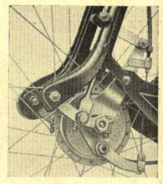
Country churches are often inaccessible by public transport. This Bown moped has brought its rider right to the lych-gate cleanly, and in good time. (Above) The trailing-link front suspension of the Bown, seen with its light alloy shielding removed. Note the parallel torque linkage for the brake arm.
