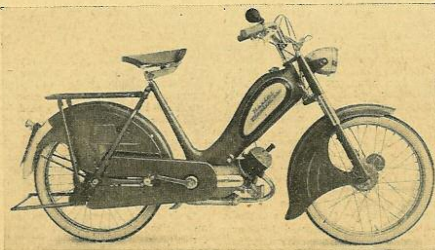
The generously valanced mudguards are displayed to advantage here, as is the sensible chain-guard. Induction is via a rotary valve, as the carburettor mounting position indicates. The sturdy carrier is a useful fitting.
